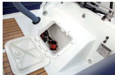
Bilge and pump access
