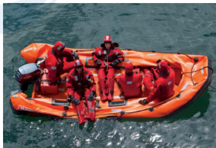
Insubmersible: Even with all its compartments deflated, the boat conserves its buoyancy with crew and equipment.
